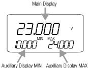
The main display appears immediately after the multimeter is switched on, but the auxiliary displays have to be activated by pressing the DATAICLEAR key (except for position M $\Omega$ @...V, where the auxiliary displays appear immediately upon selecting the function).
